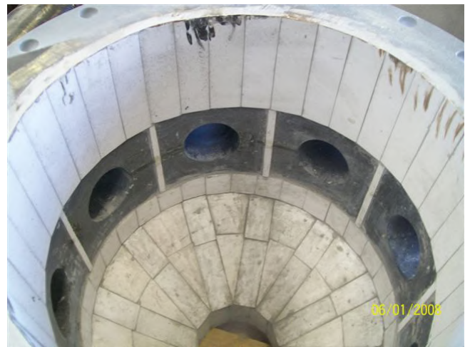
HMA distributor with full SiTech arms that extended into the main body with a radius plate as a one piece design
