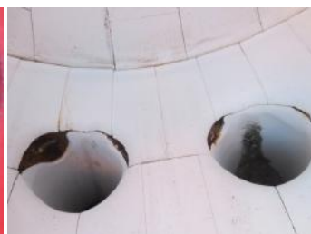
Alumina Ceramic Lined after 1600 hours
