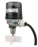
types of equipment simply will not fit. Its principle of operation is simple ... a slow speed motor rotates the paddle when no material is present. Then, when material comes into contact with the paddle, the paddle stops and an alert – such as a light or hom – will notify the operator the bin is full. When the bin is emptied, the paddle again begins to rotate, alerting the operator that a refill is necessary.
