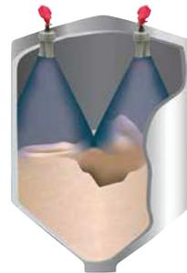
mounted in strategic locations to account for surface variations across the material surface. The software synchronizes the level data from all sensors to create a single 3D image and calculate bin volume.
