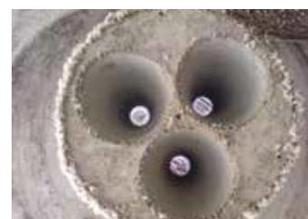
Exterior of the sensor is coated with dust, while self-cleaning properties keep the transducers clean and functional.
