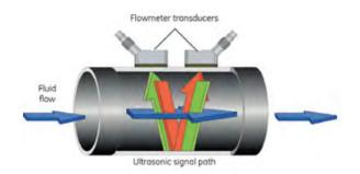
With transit time flow measurement, two transducers serve as both ultrasonic signal generators and receivers. When mounted on a pipe, they are in acoustic communication with each other, meaning the second transducer can receive ultrasonic signals transmitted by the first transducer and vice versa.
