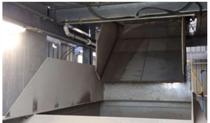
4 x Bisalloy plates fitted to left hand side hopper.
