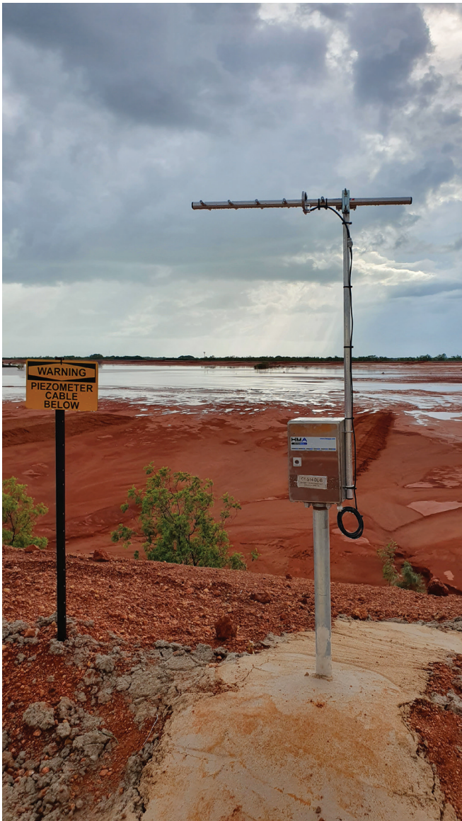
Node (data logger with sensor) in a protective enclosure, with Yagi antenna.
