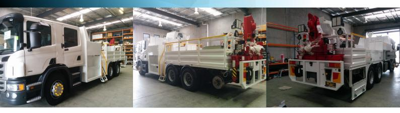
The Scania P 310 is raised up using the PTO to drive a hydraulic pump that pushes the rail guidance system (train wheels) into contact with the track. The front end of the truck is raised relative to the rear, as the rear drive tyres remain partially in contact with the rails to provide forward motion, even though the rear rail guidance wheels are in touch with the track. That way the truck can use its powertrain to move, Pike explains.
