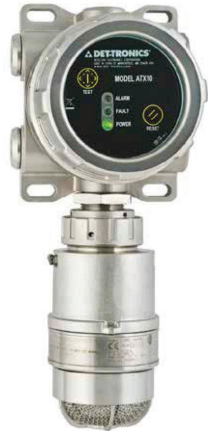
Above: Acoustic gas leak detectors work by recognizing the unique sound "fingerprints" of various gases. However, the sound and impact of blowing sand particles can create nuisance ultrasonic noise and lead to possible fault conditions in windy desert environments. The Det-Tronics FlexSonic detector shown above uses a foam filter to eliminate ultrasonic noise due to particle impact with the microphone.
