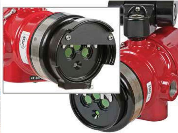
Above: Heavy wind, rain or snow can lead to weather-induced fault conditions for flame detectors because infrared radiation is absorbed by water molecules. To minimize the accumulation of moisture or condensation on detector optics, look for IR detectors with lens heaters and device shielding (as shown on the Det-Tronics X3301 Multispectrum IR detector).
