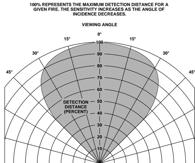
Figure 7—Detector Cone of Vision
