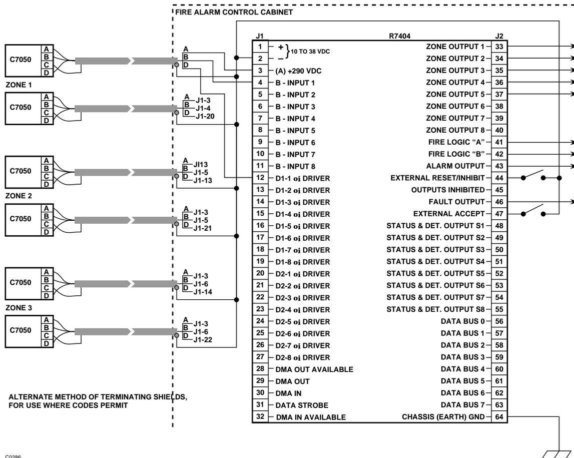
Figure 23—Typical System - Six Detectors in Three Zones
