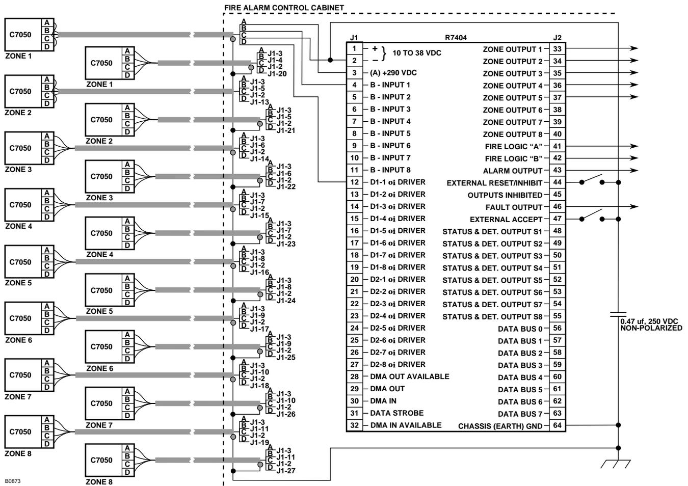
Figure 24—A Typical System – 16 Detectors in 8 Zones
