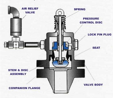
The valve seat is welded into the valve body and its flexible design compensates for distortion caused by thermal expansion. The sealing surface of the seat is stellited to minimise wear and reduce maintenance to the valve
