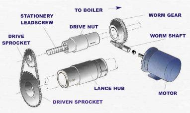
Where the element has to be rotated as it travels, a chain and sprocket drive arrangement is used to rotate the lance hub. Where the element is of the non-rotating type, the hub drive arrangement is omitted.
