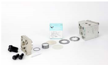
Gasket kit with gauge glass — 1050 psi; Ruby mica – retorquing required 24 hours after installation
