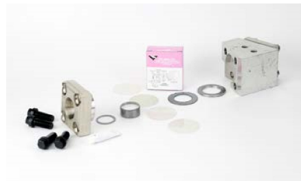
Gasket kit with gauge glass — Ruby mica – retorquing required 24 hours after installation
