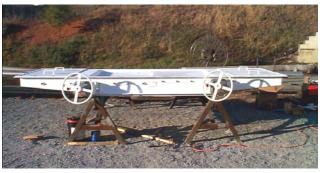
Rack and pinion gates are used generally as maintenance gates ahead of feeders and other equipment. Due to their simple construction, rack and pinion gates can be relied on to operate after months of inactivity. This is especially important in powerhouse and industrial applications.
