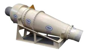
HMA Wear Solutions supplies cyclone components in a range of abrasion resistant materials such as Alumina Tiles, Alumax Monolithics, SiTech and 27% Chrome. We can also offer Aerotech, a ceramic bonding that provides a more consistent
