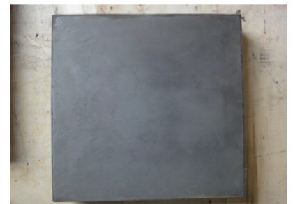
SiSiC bonded with Rubber
